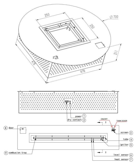
1, Before connecting electronic power to the burner, close the tank door well.
